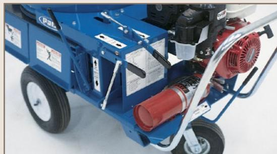
All controls are grouped together for convenient, easy operation. A (Class ABC Rated) fire extinguisher is standard equipment.
